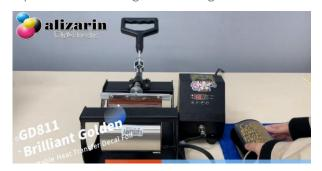
step4. Transferred by Cup heat press machine with 165°C and 120 second
